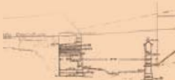
Cross section of the right salient caponier, escarp and counterscarp and magazine casemates
