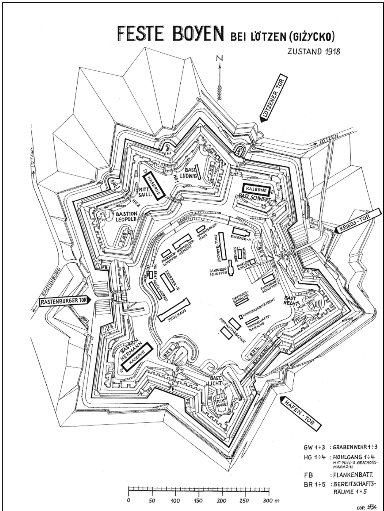
Fig. 59: Giżycko. Boyen fortified complex. Layout plan of the installation as a whole. Redrawn by Ernst Ludwig von Aster in 2006. Many of the buildings shown on the parade either no longer exist or are in ruinous condition.
